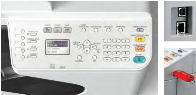
Handle multiple functions with the easy-to-use control panel. Scan to USB drives and other portable devices. Just plug in, and go. Network connectivity and USB 2.0 come standard.
